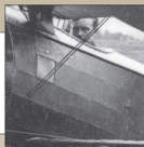
^ Small inspection window C6 detail from the Clayton & Shuttleworth built Sopwith Triplane N5364 as seen on page 15.
