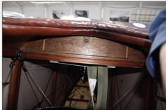
Storage locker at rear of cockpit (A13). Note the method of attaching the modern 4 point safety harness shoulder straps. The usual safety belt arrangement for RFC aircraft during WW1 was the wide 'waist belt' (P5) & (P6).
