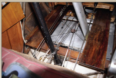
The bracing wires and control cables make for a rather cluttered appearance between the foot boards (F14) and empty shell chute (A8). Note the aluminium and linen areas of the fuselage bottom.
